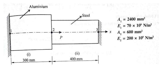
2. The stepped bar is subjected to an increase in temperature, .Use elimination method for Treatment of boundary conditions. Determine Nodal displacements and element stresses. Solve the problem using ANSYS APDL and plot the table containing results from software solution and hand calculation solutions and check for accuracy. Also submit contour plots.
